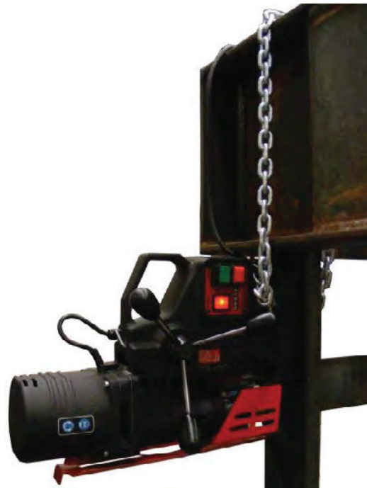
An example of a safety chain/strap use.
